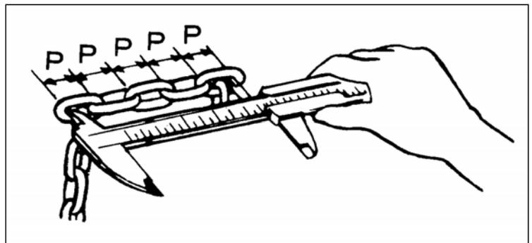
Fig 7 Checking chain dimensions
