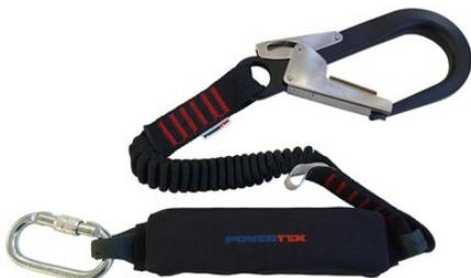
The Powertex FL-1 flexible lanyard is equipped with a shock absorber and is approved for 140 kg use. This lanyard is elastic, allowing it to stretch per the user's movements. The lanyard is securely sewn to a shock absorber pack, which includes a screw gate steel carabiner for attachment to a harness. Sewn-in double-action aluminum scaffold hooks provide reliable anchorage on the other end of the lanyards.
